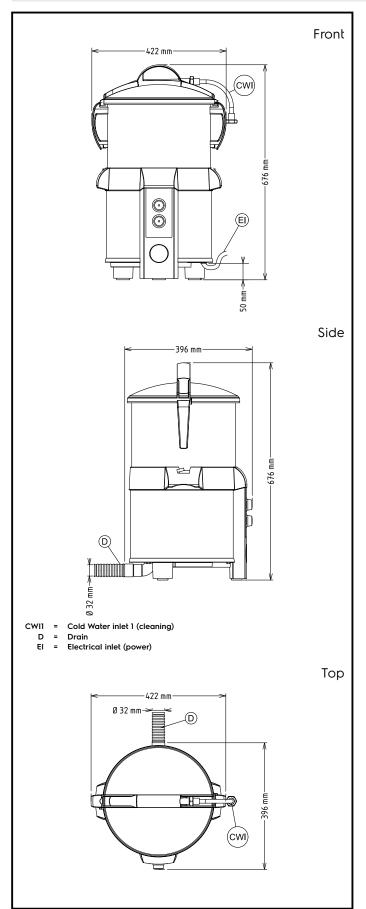
**Electric** Supply voltage: 601492 (T8EFB) 220-240 V/1N ph/50/60 Hz
